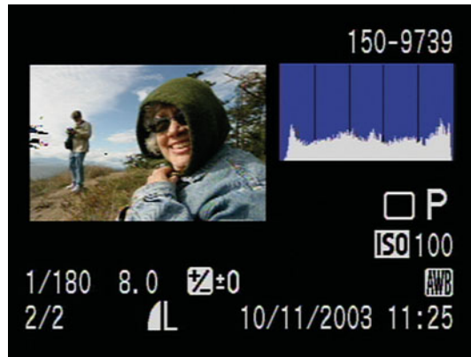
FIGURE 5.35 As you'll learn in Chapter 8, having a camera that can display a histogram is an invaluable aid for using your camera's manual exposure features.
